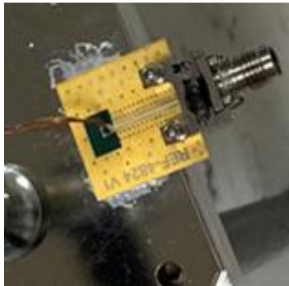
Figure 14. Test fixture used for the power handling test of the high frequency SMT RF termination
