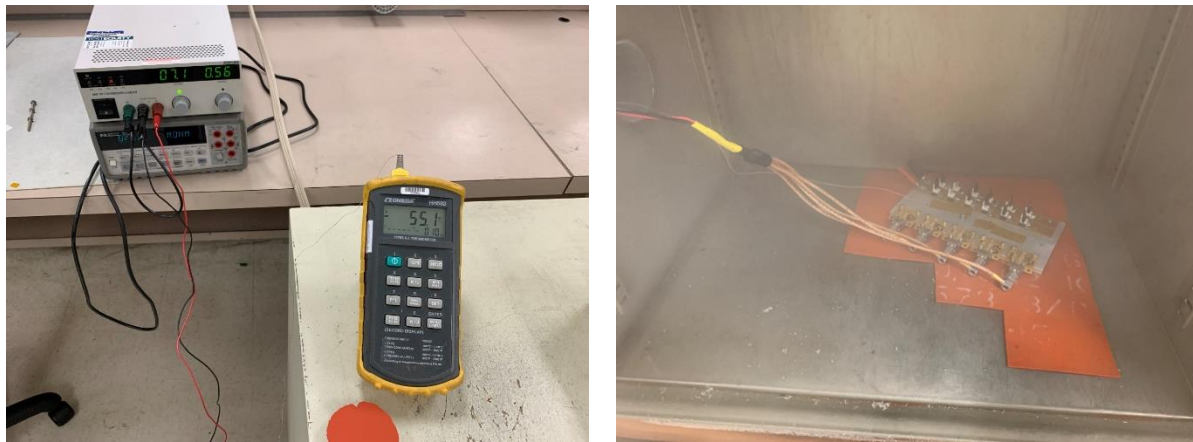
Figure 27. Test setup for low temperature operation test
