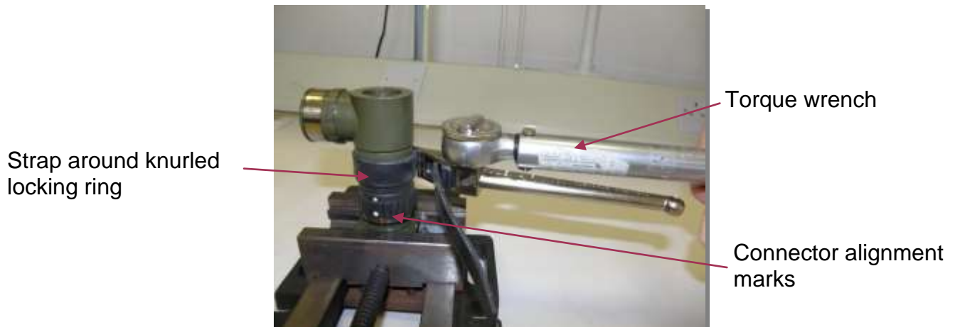
Figure 13: Tightening backshell using strap wrench/torque wrench combination
