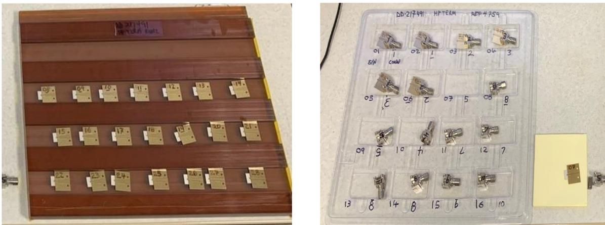
*Figure 24. Group A inspection lot: test fixtures without the connectors installed (left), test fixture with the connectors installed (right)*
