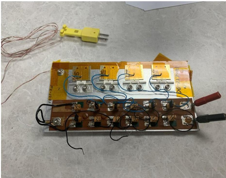
*Figure 27. Burn-in fixture for the bake test*
