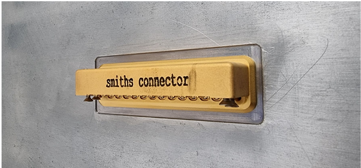
Nexus Connector – Fitted to test panel (tested without PCB fitted)
