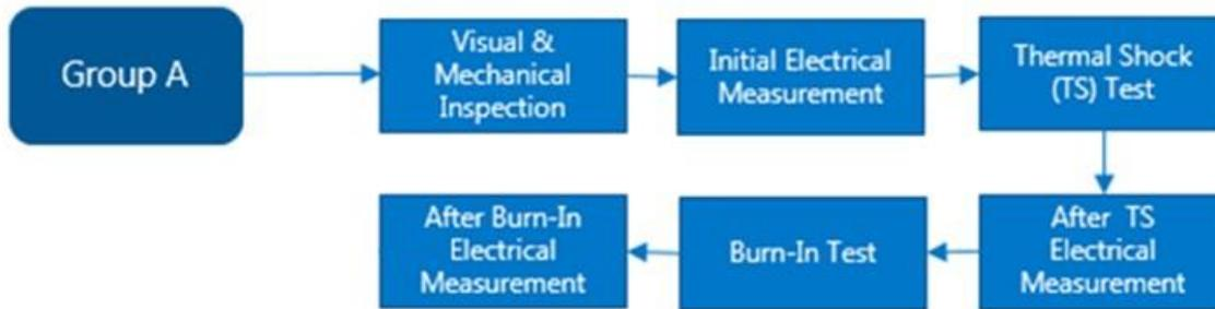
Figure 6 – Flowchart of Test Procedure
