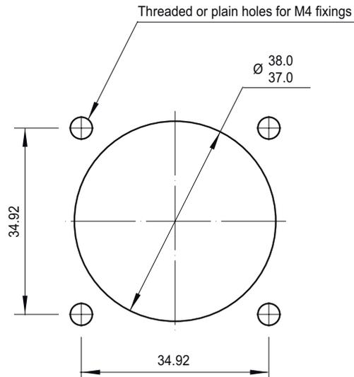
Recommended maximum panel thickness = 5.0 mm. If panel is more than 3.0 mm thick then fixing screws may need to be recessed to give clearance for mating connector.
