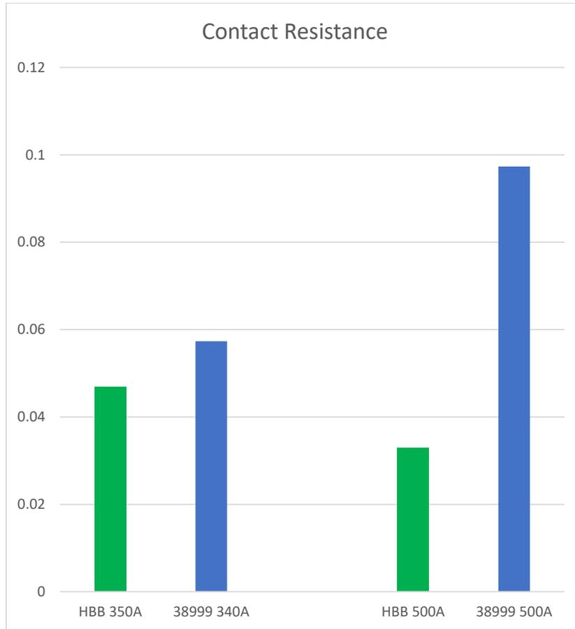
Figure 10: Chart Showing Average Contact Resistance of HBB Family vs Competitor
