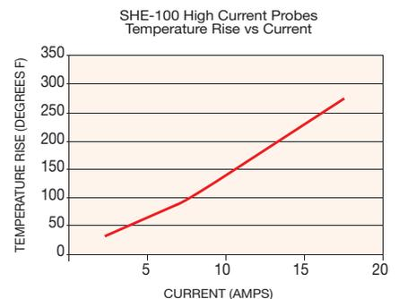
1. For SH-100 Series only 2. Smiths Interconnect's current ratings are defined as the maximum current at which the temperature rise of the probe does not exceed 144°F (80°C) for a single probe in free air at ambient temperature for one hour. Dimensions are in inches (mm) | All specifications are subject to change
