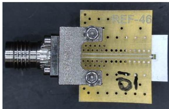
Fig. 4. The test fixture used to test the presented RF termination
