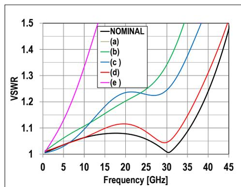
Fig. 3. Simulated electrical performance for the scenarios shown in Fig 2 (a) – (e)
