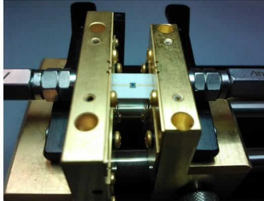
Fig. 9 Anritsu Universal Test Fixture (UTF) used in many high frequency test applications
