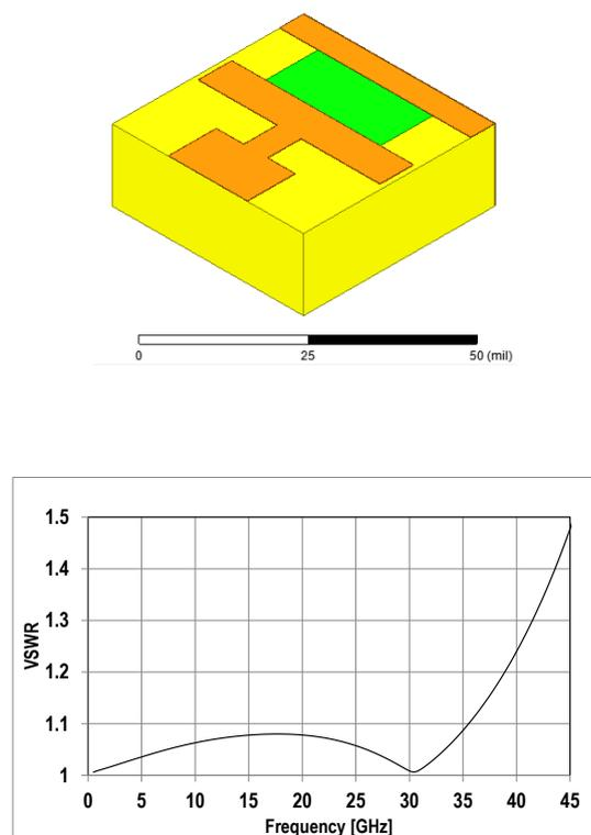
Fig. 1. Surface mount RF termination: (a) model in Ansys HFSS, (b) simulated nominal RF performance (VSWR).
