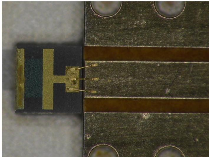
Fig. 8. Properly installed RF termination on the test fixture; good correlation between the simulated model and the prototype
