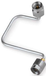
Care should be taken to avoid over-bending test cables beyond minimum bend radius guidelines. Over-bending can force cable center conductor off-center and can force the outer conductor out of round even to the point of kinking and fracture. Over bending results in degraded IL and SWR performance. It should also be noted that coiling cables at small diameters could force connector center-pins to protrude beyond required interface dimensions.
