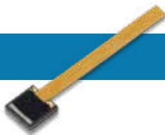
Our exclusive line of CVD Diamond chip terminations offers a unique combination of extreme high power ratings in very small packages. These terminations may be used in applications from DC to 26.5 GHz and are ideal for military and space applications because of their high power capability, broad frequency response and small, light-weight package size. These terminations are available in easy to mount tab and flange mount units.
