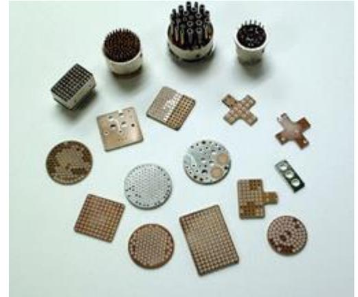
Smiths Interconnect uses a thin wall ground plane to house the filter elements. The ground plane is captured between halves of the connector shell to provide mechanical retention as well as electrical contact. Thermal stress from the connector shell is not transferred to the capacitor arrays due to a gap between the outside diameter of the ground plane and the inside of the shell. Stress from the contacts is eliminated through the use of a block of epoxy on either side of the capacitors.
