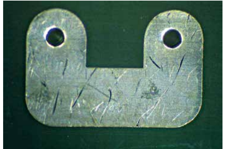
PHOTO OF CONTACT SURFACES AFTER TESTING FOR BIAS BALL CONFIGURATION
