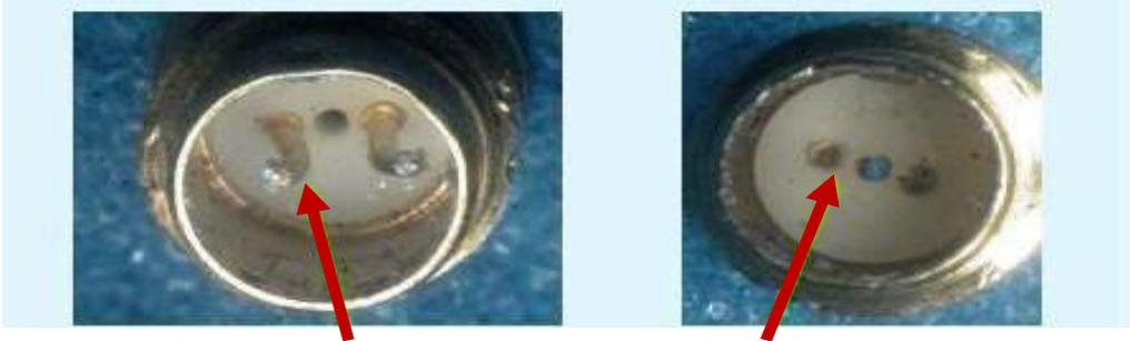
Fig. 1 – Standard Gender (Pin Exposed) Pin Damage
