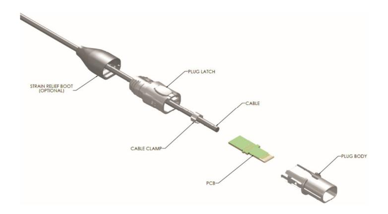
**Step 2:** Trim and strip cable and wires to length.
