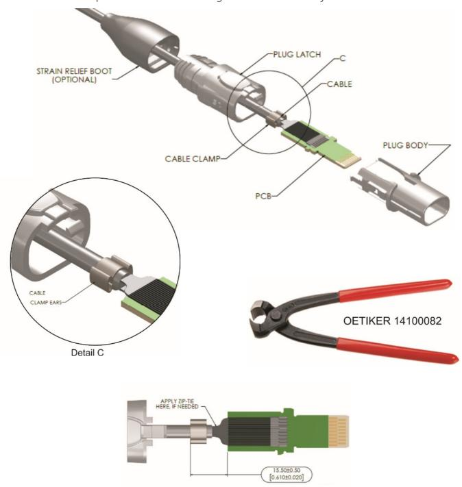
**Step 6:** Position PCB as depicted below, assuring the ears of the PCB are oriented relative to the top of the plug body in images below.
