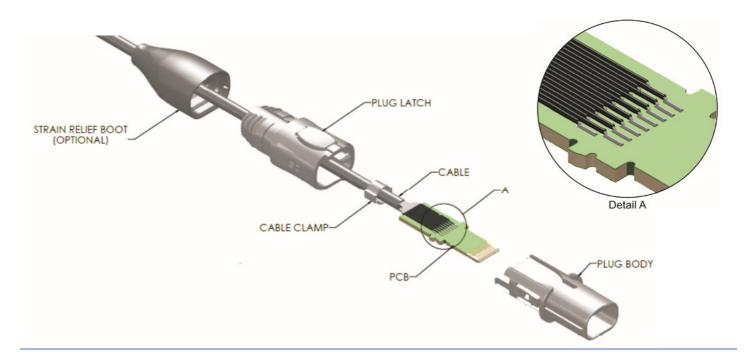
**Step 4:** Apply Epoxy over the soldered wire-connections and fully cure before moving onto the next step
