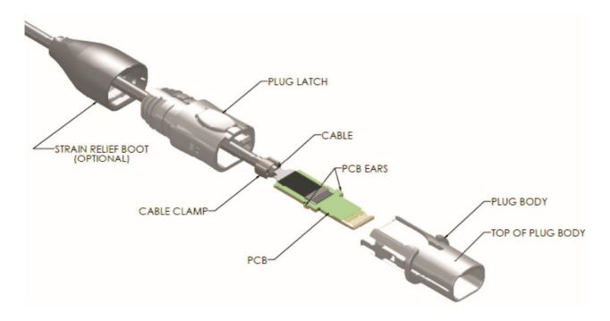
Install PCB into plug body until both ears of PCB snap into place
