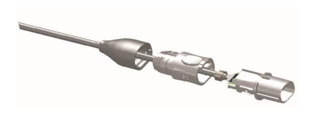
**Step 7:** Align plug latch alignment features with plug body alignment features and slide plug latch down cable until it bottoms out on the body and snaps into place. Latch alignment features may need a slight compression to allow successful snap installation.
