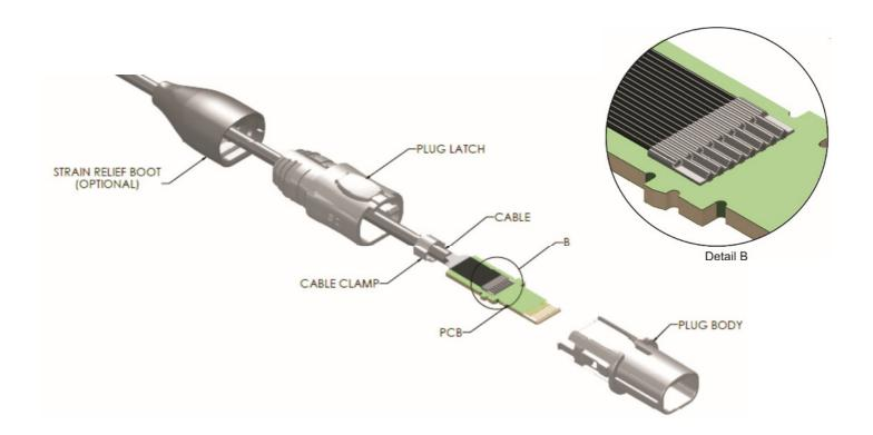
**Step 5:** Using OETIKER PN 14100082, compress cable clamp ears in place as depicted below. Cable clamp shall be located as shown in the images below.
