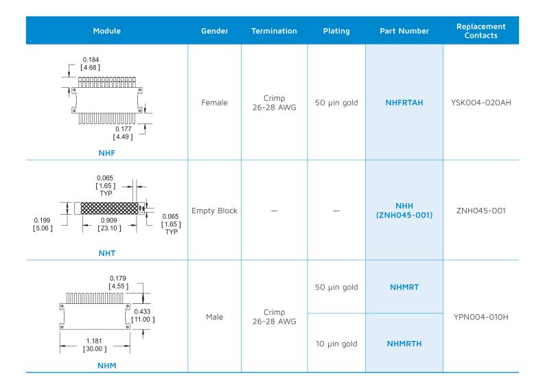
Notes: 1. Male contacts are shrouded in the insulator, female mounts in the plug frame are suggested. 2. Crimp contacts will be shipped unassembled. Dimensions are in inches [mm].
