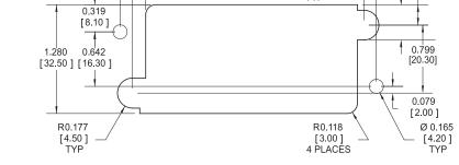
Notes: 1. 59.0 oz. in. torque for mounting. 2. Refer to individual frame type for standard length. Dimensions are in inches [mm].
