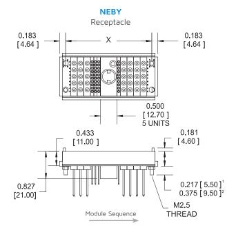
Notes: 1. Standard mounting stud length. 2. For thicker chassis, this longer mounting stud length can be selected by adding the modification code "-479" to the end of the connector part number. Dimensions are in inches [mm].
