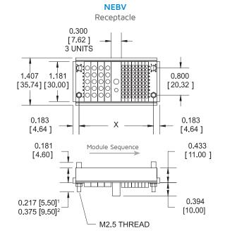
Notes: 1. Standard mounting stud length. 2. For thicker chassis, this longer mounting stud length can be selected by adding the modification code "-479" to the end of the connector part number. Dimensions are in inches [mm].
