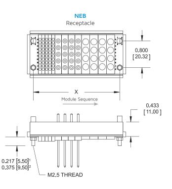
Notes: 1. Standard mounting stud length. 2. For thicker chassis, this longer mounting stud length can be selected by adding the modification code "-479" to the end of the connector part number. Dimensions are in inches [mm].
