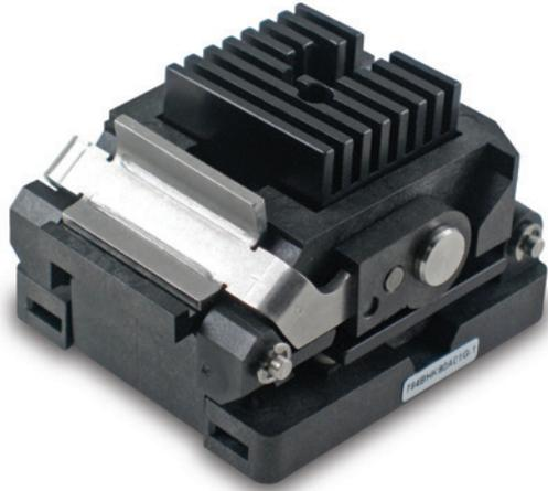
The K-Series socket is designed to apply flat even pressure on the DUT with a secondary lever once the lid has been closed. This is to ensure that the platen does not skid across the top of the device when closing the lid potentially marking the device. This is especially important for exposed die products, or automotive applications where appearance is part of the pass/fail acceptance criteria post test.
