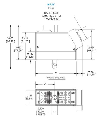
Notes: 1. Frame JY mates with NEBY or NEPJY. 2. Protective dust cover for plug only part number: ZMP0025-XX (XX = number of modules). Dimensions are in inches [mm].
