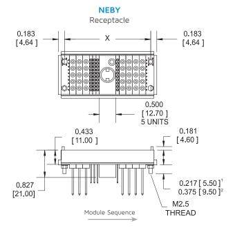
Notes: 1. Standard mounting stud length. 2. For thicker chassis, this longer mounting stud length can be selected by adding the modification code "-479" to the end of the connector part number.
