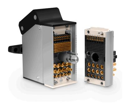
Smiths Interconnect's N Series high density, modular rack and panel connectors employ a do-it-yourself system based on the principle of building blocks. The N Series system is composed of two elements: modules and frames. Modules of various styles and contact types, including signal and coaxial, can be combined into custom arrangements within a single connector frame. This allows the user to build a connector that addresses and fulfills their exact requirements with off-the-shelf components.
