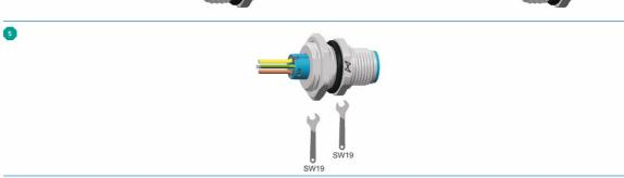
Mounting arrangement for straight receptacle and panel feed trough
