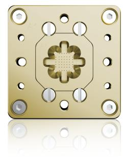
The semiconductor test industry has traditionally used spring pin technology for BGA, LGA, QFN, and QFP devices, while the cantilever scrubbing contact design has been used in peripheral segments to remove surface oxides and contaminants. However, the vertical spring probe technology used in the array segment allows for a dense population of individual contacts in the array with more Z-axis compliance.
