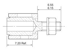
Style AM Non polarised guide socket. Vertical mounting.
