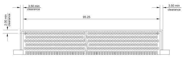
303 way showing typical clearance dimensions (applies to all  $90^\circ$  styles)
