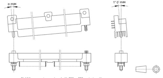
$\alpha$  = 0° 11' for connectors equipped with 220 or 236 contact positions.  $\alpha$  = 0° 07' for connectors equipped with 316 contact positions.
