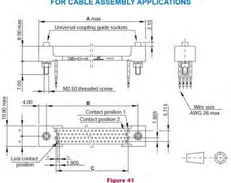
**Dimensions in width** Contact A В C positions (mm) (mm) (mm) 42 37.210 29.210 19.050 82 56.260 48.260 38.100 110 69.595 61.595 51.435 126 77.215 69.215 59.055 158 92.455 84.455 74.295 174 100.075 92.075 81.915
