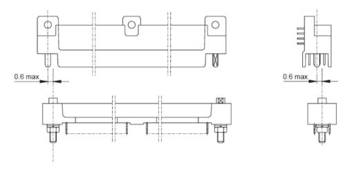
for connectors equipped with 220, 236 or 316 contact positions.
