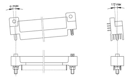
$\alpha$  = 0° 25' for connectors equipped with 42, 82, 110, 126, 158 or174 contact positions.
