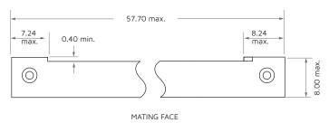
Please note the 048 way is the only non-symmetrical connector in this range. Therefore care should be taken to ensure correct identification code.
