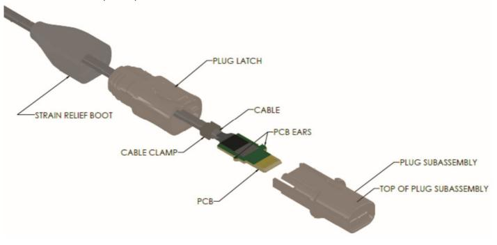
Install PCB into plug subassembly until both ears of PCB snap into place.
