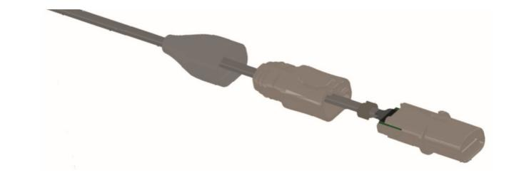
**Step 5:** Align plug latch alignment features with plug subassembly alignment features and slide plug latch down cable until it bottoms out on plug subassembly and snaps into place. Latch alignment features may need a slight compression to allow successful snap installation.
