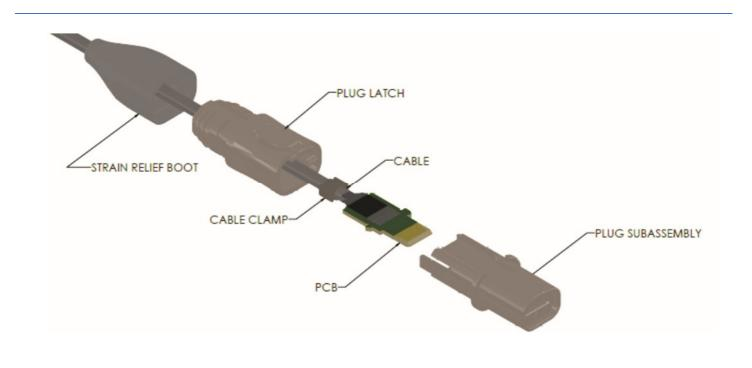
**Step 4:** Position PCB as depicted below, assuring the ears of the PCB are oriented relative to the top of the new plug subassembly as depicted in images below. Install PCB into plug subassembly until both ears of PCB snap into place.
