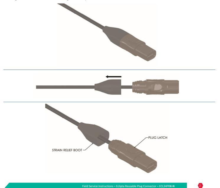
**Step 2:** Using tweezers or equivalent, disengage both latches from plug subassembly and slide plug latch back down the cable.
