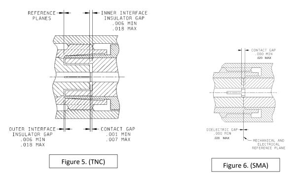
You can see by the two interfaces above that there is a much shorter path from center conductor to outer conductor in the SMA design, than in the TNC design. In addition, the TNC design has insulators that fit one inside the other. This increases the conductive path from center conductor to outer conductor and therefore increases the power capability.
