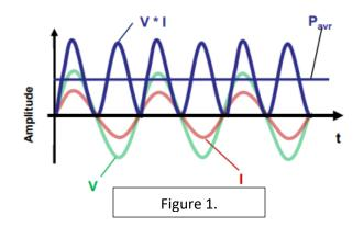
So, what are these variables that effect power in our cables as mentioned earlier? The first one is <u>Frequency</u>. The main premise being as the frequency increases, the power decreases. The simple reason is that due to the laws of Microwave Signal Transmission, higher frequencies are supported and transmitted in smaller cables, and the smaller the cable, the harder to dissipate the heat resulting in power loss.
