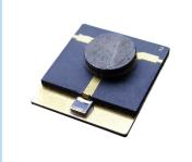
The I7696/A, I94118/A and I104142/A low power microstrip isolators were designed to be in a next generation GEO HTTP satellite and used in a filter demultiplexer application. These low power microstrip isolators are intended to be used within a hybrid construction and must be wire bonded into the user's circuit. Key performance requirements include electrical performance and operating bandwidth.
