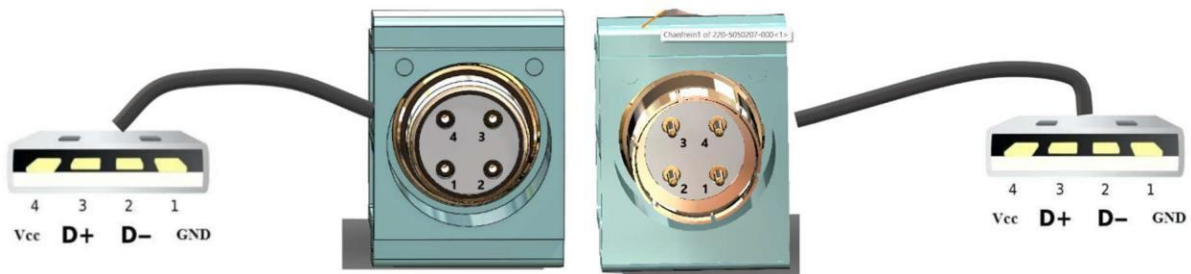
Figure 12. USB 2.0 standard cable and wiring diagram
