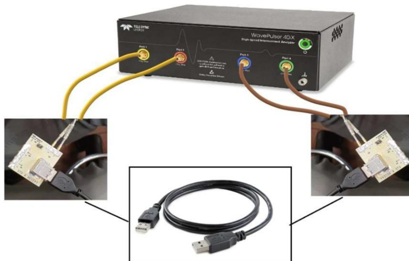
Figure 19. Experimental setup for measuring USB 2.0 standard cable electrical performance
