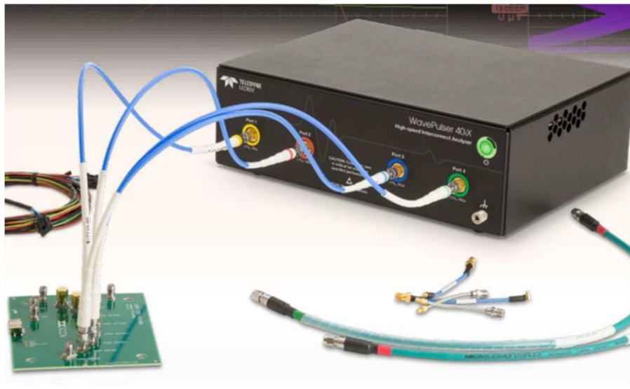
Figure 15. Example of experimental setup using WavePulser 40iX Interconnect Analyzer
