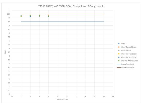
Figure 10 - TT910.0SMT DC Attenuation Group A and B Subgroup 2
