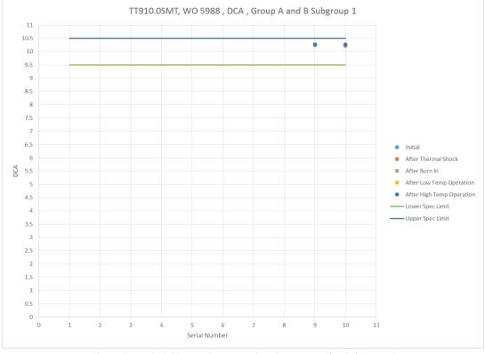
Figure 9 - TT910.0SMT DC Attenuation Group A and B Subgroup 1
