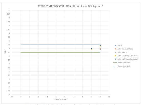
Figure 6 - TT906.0SMT DC Attenuation Group A and B Subgroup 1
