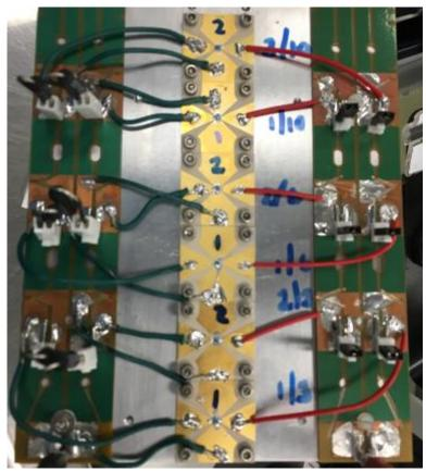
Figure 2 - Burn in Fixture FX-1263
