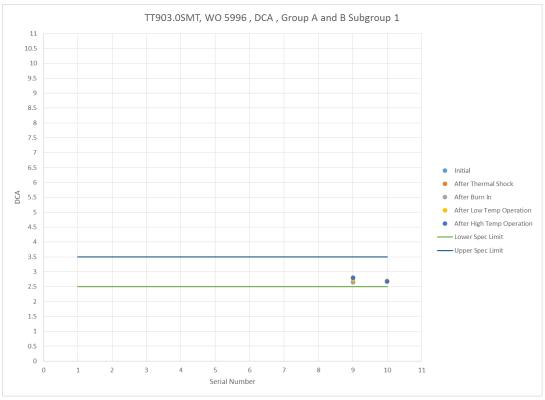
Figure 3 – TT903.0SMT DC Attenuation Group A and B Subgroup 1
