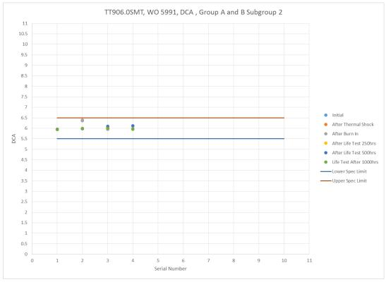
Figure 7 - TT906.0SMT DC Attenuation Group A and B Subgroup 2
