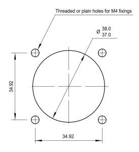
Recommended maximum panel thickness = 5.0 mm. If panel is more than 3.0 mm thick then fixing screws may need to be recessed to give clearance for mating connector.
