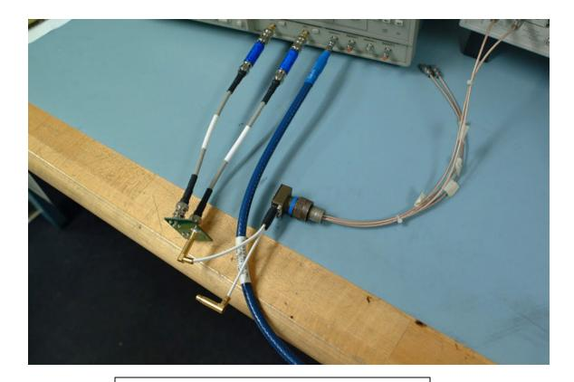
Figure 4 Test Connector and Related Wiring
