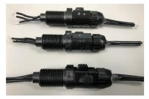
connectors were mated and unmated 200 times to assure that no substantial changes occurred. Finally, the dielectric withstanding voltage was checked on each connector pair confirming that the insulators continued to meet the design specification.
