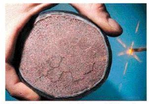
A Single optical fiber can hold as much information as this large cable containing thousands of copper wires.
