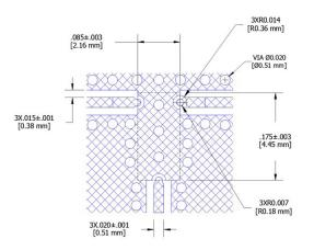
Metric dimensions for Reference only. Transmission line dimensions based on a Rogers 6035HTC substrate, 0.010" thick, 1/20z, copper both sides.
