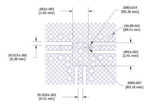
Metric dimensions for Reference only. Transmission line dimensions based on a Rogers 6035HTC substrate, 0.010" thick, 1/20z, copper both sides.
