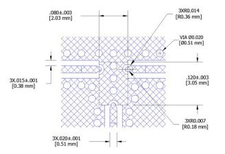
Metric dimensions for Reference only. Transmission line dimensions based on a Rogers 6035HTC substrate, 0.010" thick, 1/20z, copper both sides.
