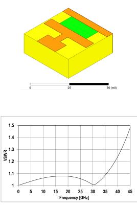
Fig. 1. Surface mount RF termination: (a) model in Ansys HFSS, (b) simulated nominal RF performance (VSWR).
