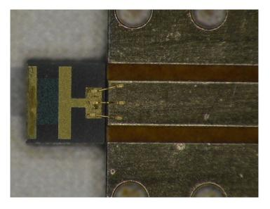
Fig. 8. Properly installed RF termination on the test fixture; good correlation between the simulated model and the prototype
