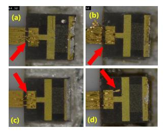
Fig. 7. Bad mounting practices: (a) poor wire bond connection to the pad, (b) air gap between the termination and the application board, (c) poor wire bond, (d) wire bond sticking out of the pad area
