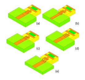
Fig. 2. Various tolerance scenarios: (a) ribbon bond (b) ribbon bond and air gap, (c) three wire bonds with significant height, (d) low height wire bonds, (e) thin application board.
