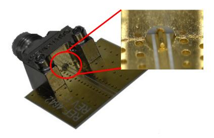
Fig. 6. Connector pin alignment on the test board
