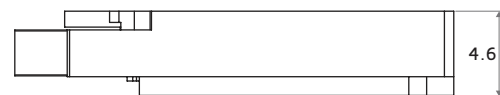
Drawing of SpaceABLE 10G SL 4TRX, 12TX, and 12RX (measurements given in mm).
