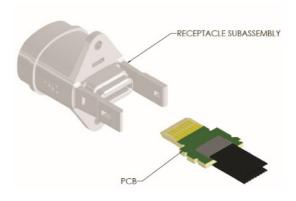
**Step 2:** Position PCB as depicted below, assuring the ears of the PCB are oriented relative to the top of the replacement receptacle subassembly as depicted in images below. Install PCB into receptacle subassembly until both ears of PCB snap into place.
