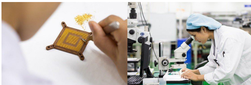
Figure 1. This image depicts a test socket being prepared for use on an ATE system. Source: Smiths Interconnect
