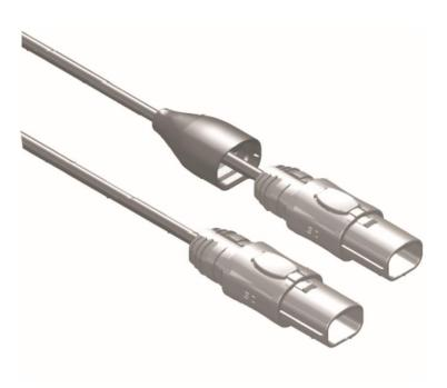
**Step 8:** If optional strain relief boot is used, align internal rib in boot with slot on plug latch, then slide strain relief boot down cable and push it onto the back end of plug latch until it fits snuggly in place. If no strain relief boot is used, over-molding is required to ensure proper cable durability.
