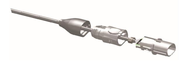
**Step 7:** Align plug latch alignment features with plug body alignment features and slide plug latch down cable until it bottoms out on the body and snaps into place. Latch alignment features may need a slight compression to allow successful snap installation.
