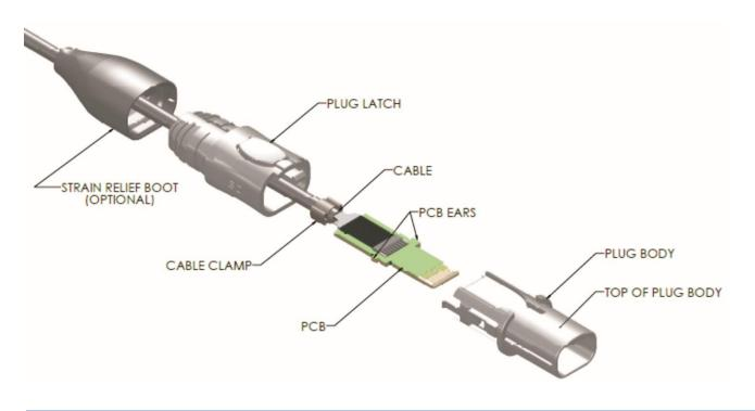
Install PCB into plug body until both ears of PCB snap into place
