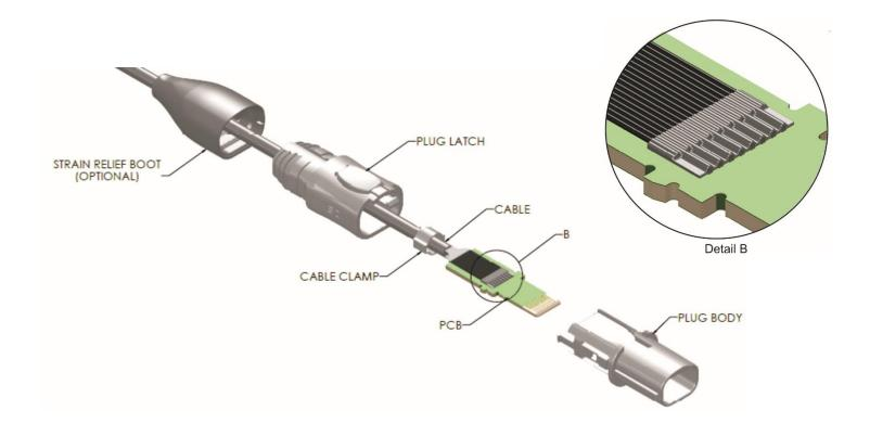
**Step 5:** Using OETIKER PN 14100082, compress cable clamp ears in place as depicted below.
