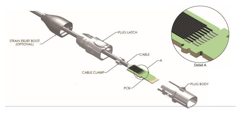
**Step 4:** Apply Epoxy over the soldered wire-connections and fully cure before moving onto the next step
