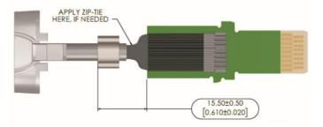
**Step 6:** Position PCB as depicted below, assuring the ears of the PCB are oriented relative to the top of the plug body in images below.
