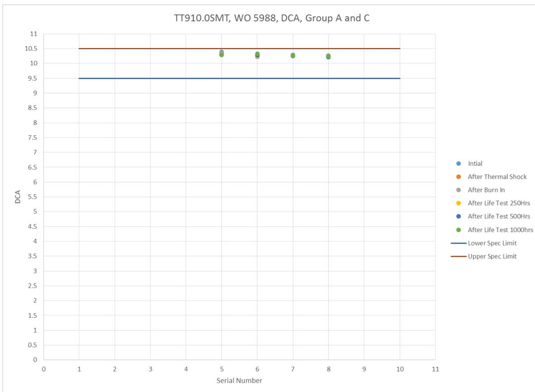
Figure 11 - TT910.0SMT DC Attenuation Group A and C
