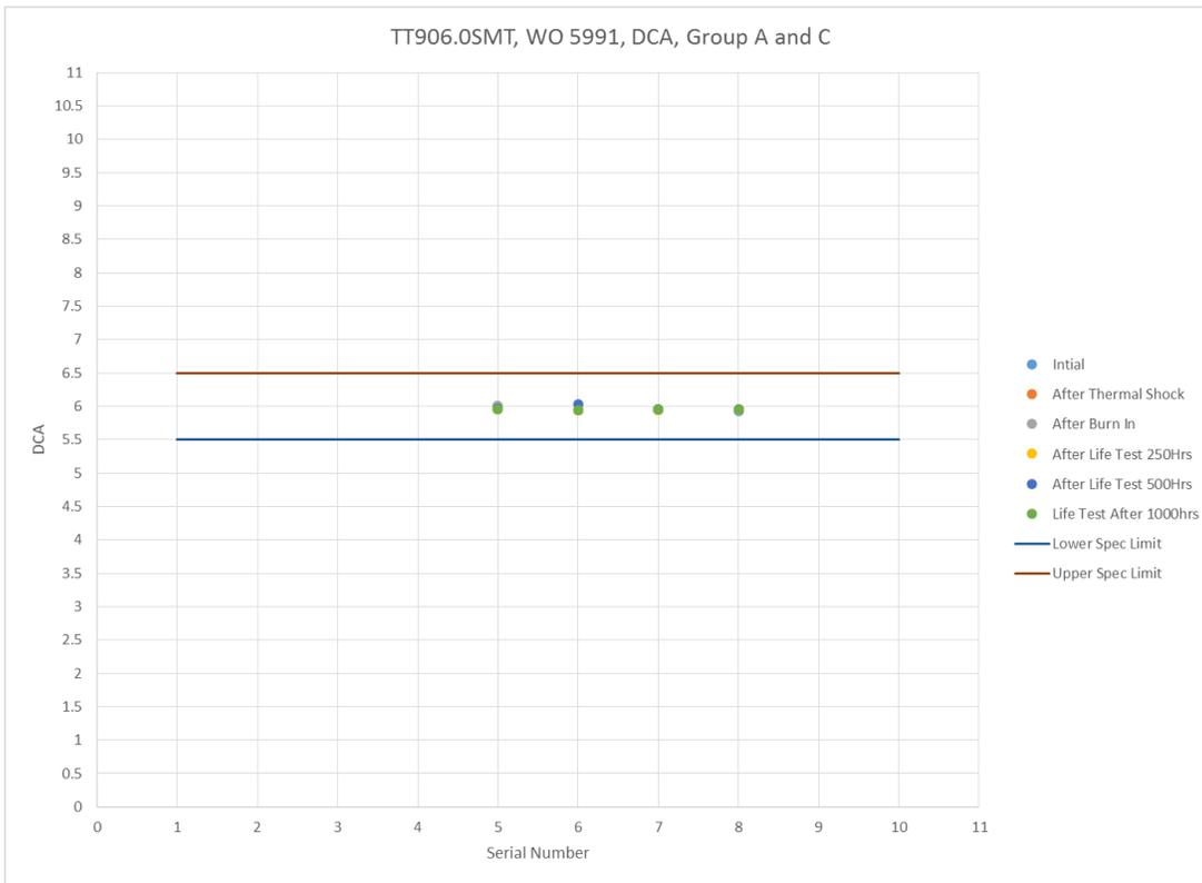
Figure 8 - TT906.0SMT DC Attenuation Group A and C
