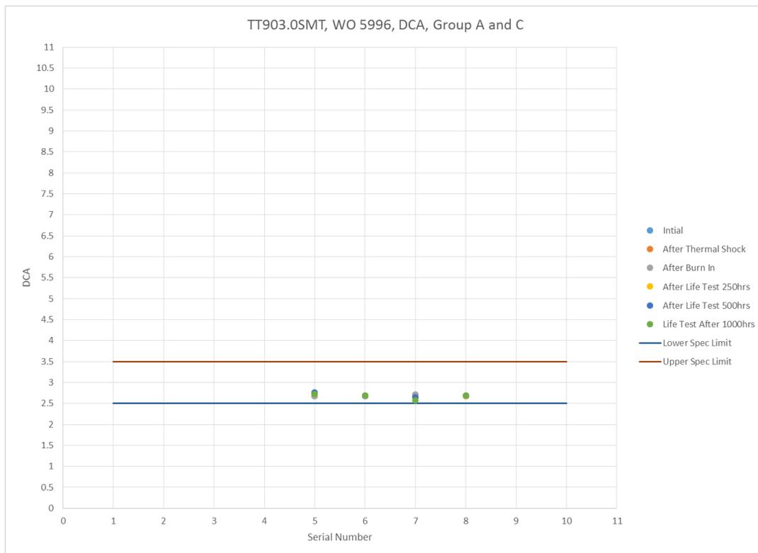
Figure 5 - TT903.0SMT DC Attenuation Group A and C
