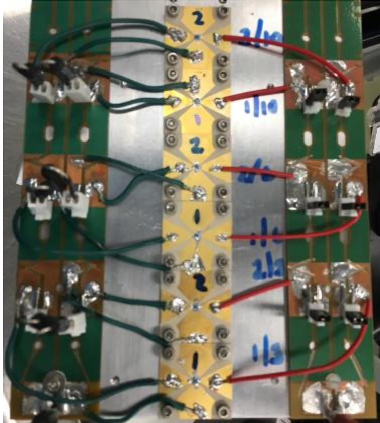
Figure 2 - Burn in Fixture FX-1263
