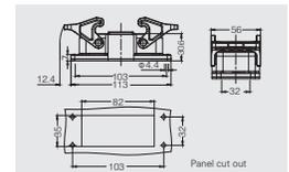
Housings, surface mounting high construction
