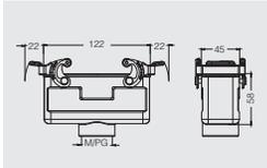
Housings, cable to cable high construction
