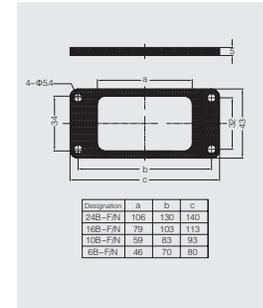
The thickened bottom gasket shown above is applicable to the regular BK housing of the same specification of H series.
