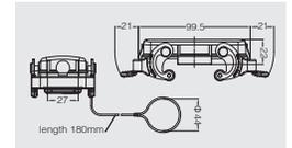
Degree of protection: IP65 1lever locking system
