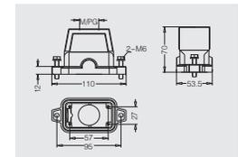
Surface mounted housings high construction
