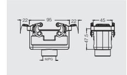
Degree of protection: IP67 1lever locking system
