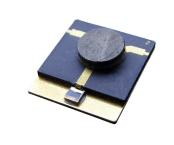
The I7696/A, I94118/A and I104142/A low power microstrip isolators were designed to be in a next generation GEO HTTP satellite and used in a filter demultiplexer application. These low power microstrip isolators are intended to be used within a hybrid construction and must be wire bonded into the user's circuit. Key performance requirements include electrical performance and operating bandwidth.
