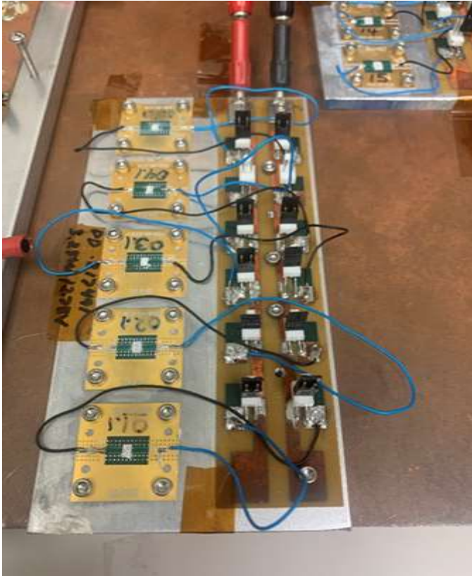
Figure 5: CRH08110505F Burn In Setup
