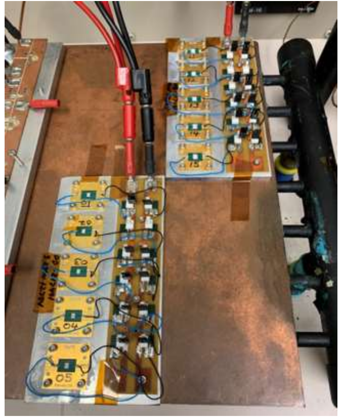
Figure 6: CRH12160505F Burn In Setup
