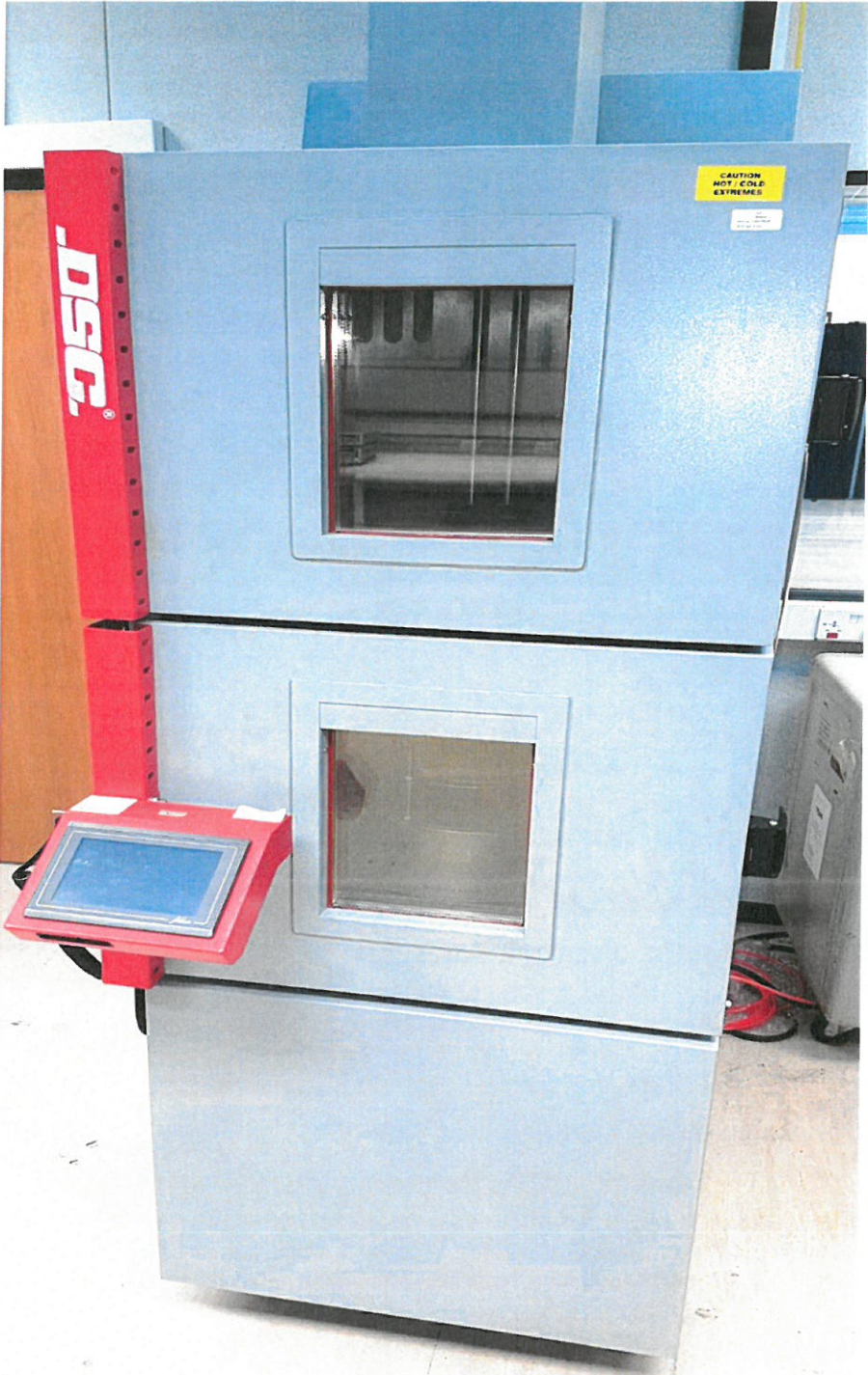
Figure 4: DSC Thermal Shock Chamber
