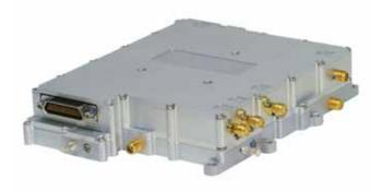
Smith Interconnect's frequency converters provide frequency translation of the input signal to a desired output frequency. They support up and down frequency translations with either fixed local oscillators (block converters), or tunable local oscillators (agile converters).
